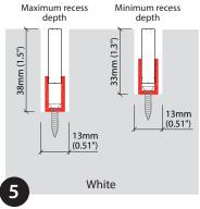
PVC channel accessory can be used to install GROOVE Light IP67 into a recessed channel at any orientation, 33mm (1.3") to 38mm (1.5") for white recess depth by 13mm (0.51") width.
