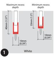
GROOVE Mini Clip accessory can be used to install GROOVE Light IP67 into a recessed channel at any orientation, 33mm (1.3") to 40mm (1.57") for white recess depth by 10mm (0.39") width.
