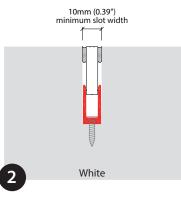
Finish slots between product and channel material with suitable filling product, such as grout, silicone or mortar.
