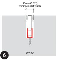
Finish slots between product and channel material with suitable filling product, such as grout, silicone or mortar.
