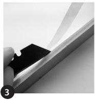
Trim masking to ensure its flush with GROOVE Light IP67 front face.
